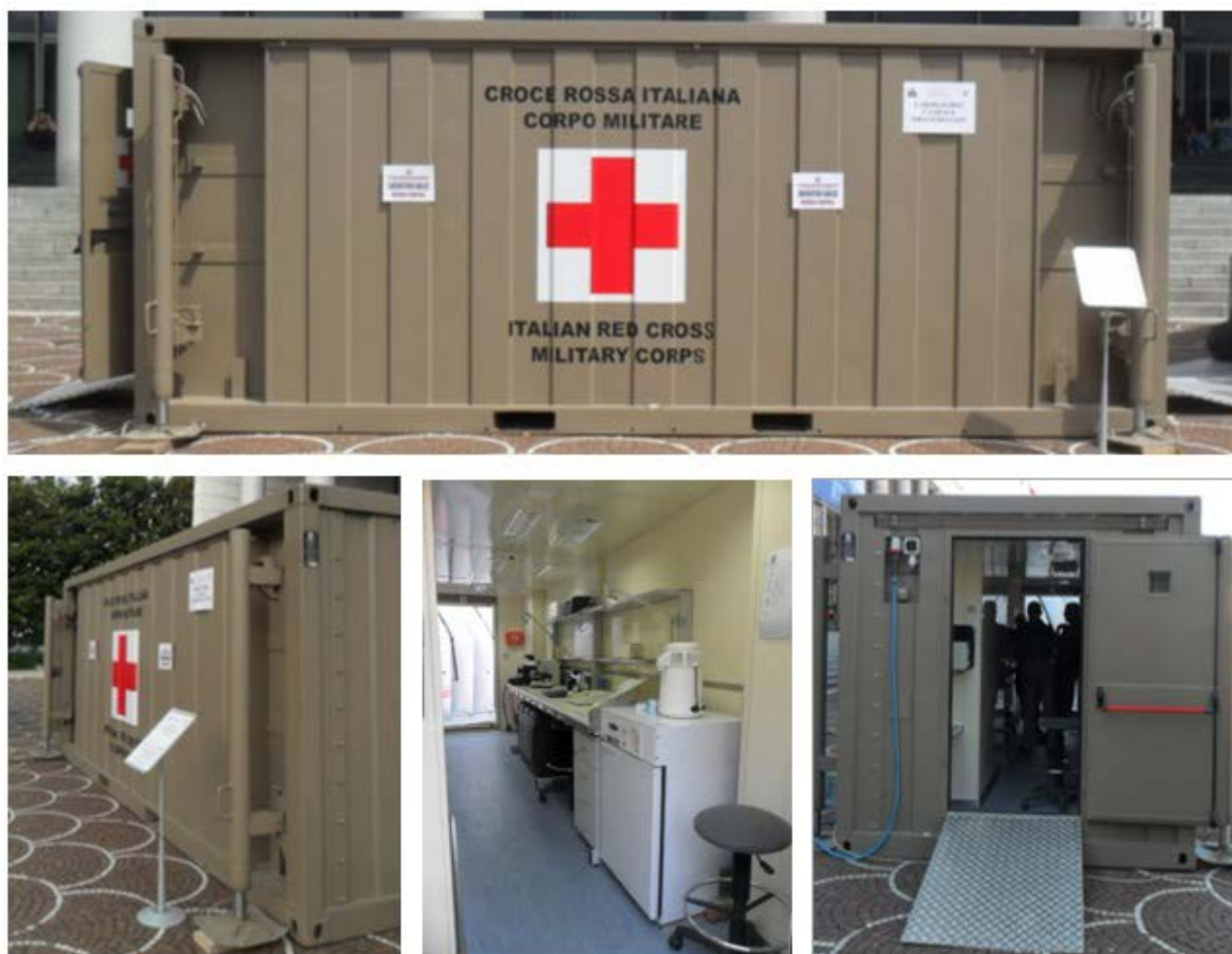
Figure 1. Outside and inside views of the sheltered laboratory of the Military Corps. This module is six meters long (upper panel). The outside view (left-bottom panel) shows details of the pneumatic positioning system. The outside-lateral view shows the entrance and power plugs (right-bottom panel). The inside view shows the position of the equipment.
